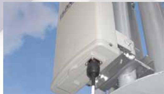
5) All LanPro wireless devices for outdoors use a network port to connect to the telecommunication equipment of the internal network. This connection through the network port of the wireless device must be protected by the plastic "waterproof connector". Similarly, the network cable must be coated for the outdoor installation. In case this cable wears down over the time, it must be replaced.
