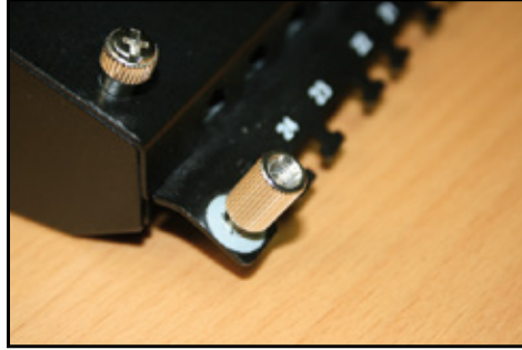
Frame Grounding post
