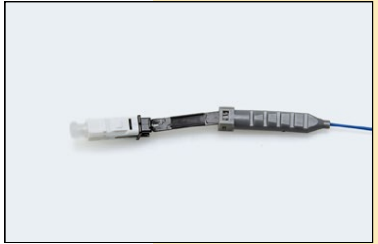
8. Assemble the boot and the cap
