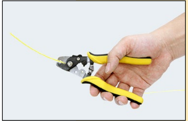
2. Strip Drop cable with a stripper
