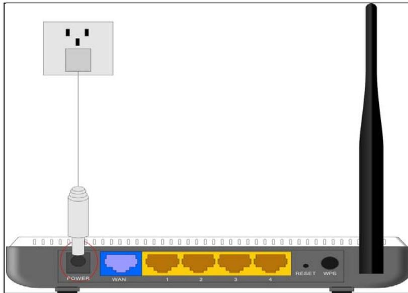
2. Please connect the LAN port of the Router to the network adapter of your computer with a cable.
