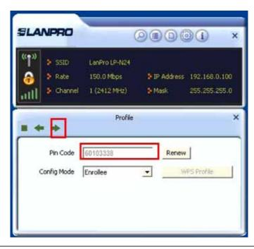
Here we take LanPro's LP-N24 as an example. First enter its WPS configuration screen, enable WPS settings and select PIN for WPS mode and then input 60103338 in the PIN code field, and then click the "Save" button. When the WPS indicator of the Router starts flashing, it indicates that WPS feature is enabled.
