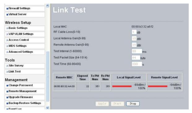
Figure: 6-2 Link test
