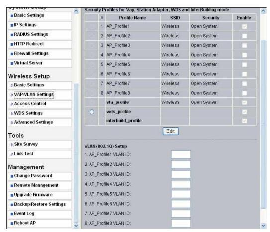
You can configure each profile by clicking "Edit". Such configuration as configuring profile name, SSID, enabling "broadcast SSID", or doing security. Figure 5-3 Security profile for Vap x
