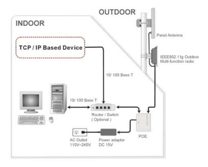
Figure 1-3 Hardware Installation Figure
