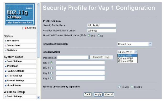
Figure 5-4 Security profile with WEP encryption
