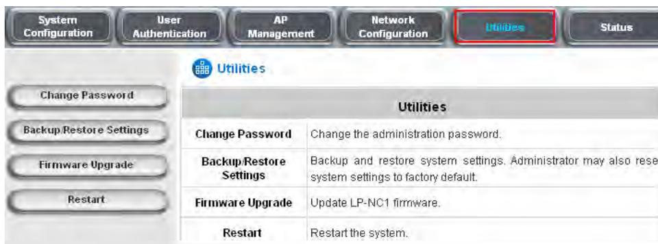
The screenshot shows the Utilities page in the LANPRO LP-NC1 web interface. The top navigation bar includes buttons for System Configuration, User Authentication, AP Management, Network Configuration, Utilities (highlighted with a red box), and Status. Below the navigation bar, there is a sidebar with buttons for Change Password, Backup/Restore Settings, Firmware Upgrade, and Restart. The main content area is titled 'Utilities' and contains a table with the following information:
