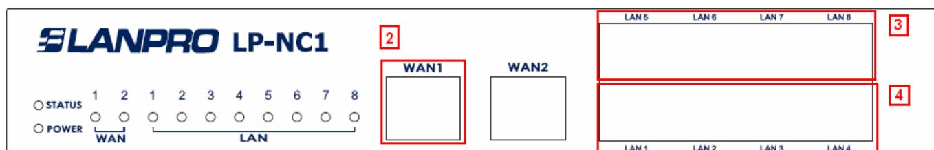
2. Connect an Ethernet cable to the WAN1 Port on the front panel. Connect the other end of the Ethernet cable to an ADSL modem, a cable modem or a switch/hub of the network. The LED of WAN1 port should be on to indicate a proper connection.
