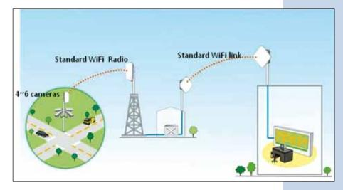
Usually a standard 802.11 Wi-Fi radio supports 4~6 cameras as the maximum, even though it has 23 Mbps effective data rate. The video quality performance is H.264 & MPEG4 without lag @ 30 fps and no mosaic.
