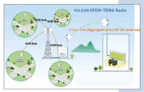
The LanPro VULCAN link easily aggregates the cameras up to  $16 \sim 20$  cameras. And the video quality supports the standard H.264 & MPEG4 without lag @ 30 fps and no mosaic.
