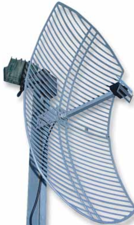
Antenna mounted in horizontal polarization mode.
