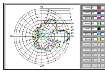
Port2-E-plane co-pol -3dB beam-width=16°
