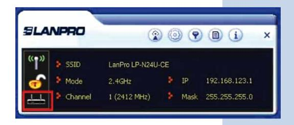
When it is switched to AP mode, the wireless adapter will automatically set its IP address as 192.168.123.1, and other clients that connected to this AP will automatically obtain the IP addresses of: 192.168.123.X(X is any integer from 2 to 254). The function buttons on the top (From L to R) are respectively Config AP, Advanced, Access Control List, Associate List, About and MiniSize, while the left column displays Turn On/Off RF, Security /No security, and AP mode icon.
