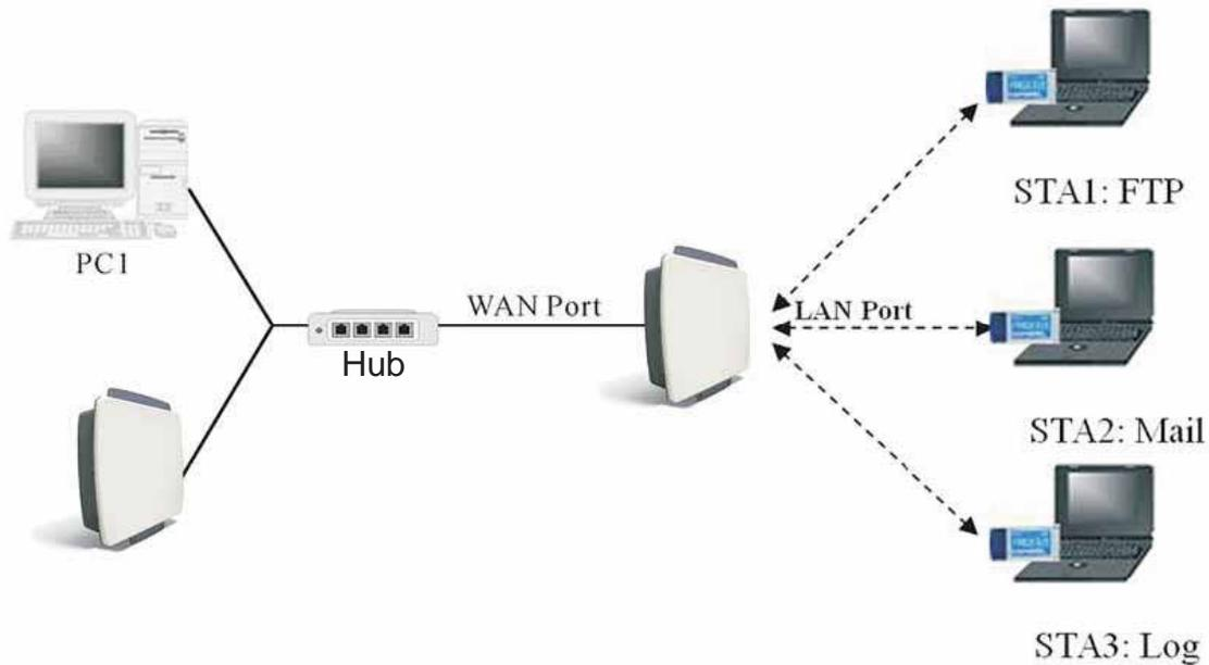
The radio (which is set as an AP) distinguishes by acting as a virtual server. This most cost-effective server virtualization technology is engineered for heterogeneous network. Please refer to the following diagram.
