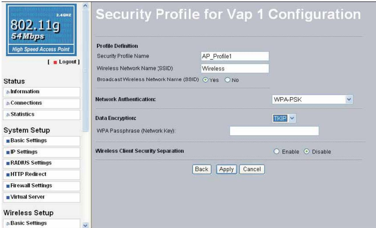
Figure 5-5 Security profile with WPA-PSK
