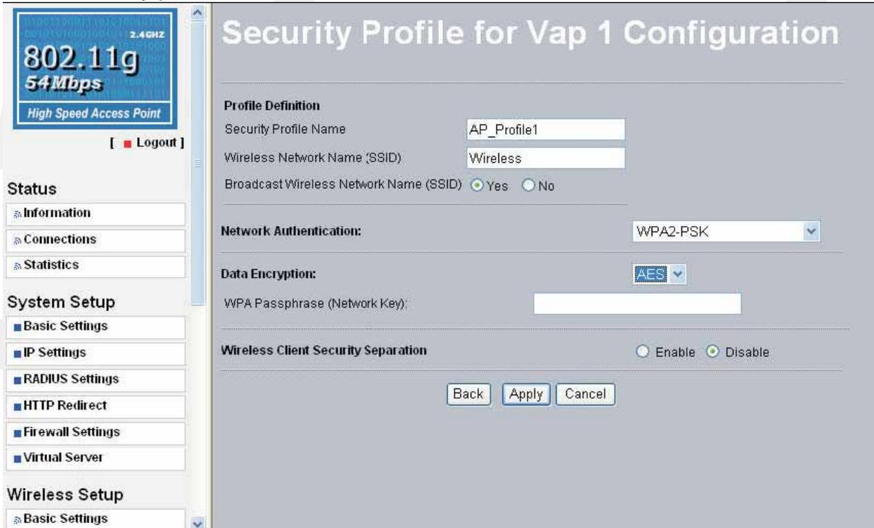
Figure 5-6 Security profile with WPA2-PSK
