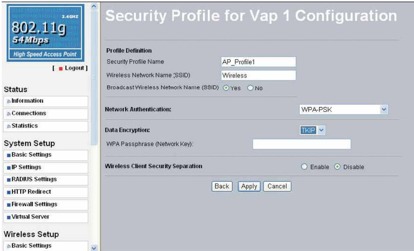
Figure 5-5 Security profile with WPA-PSK
