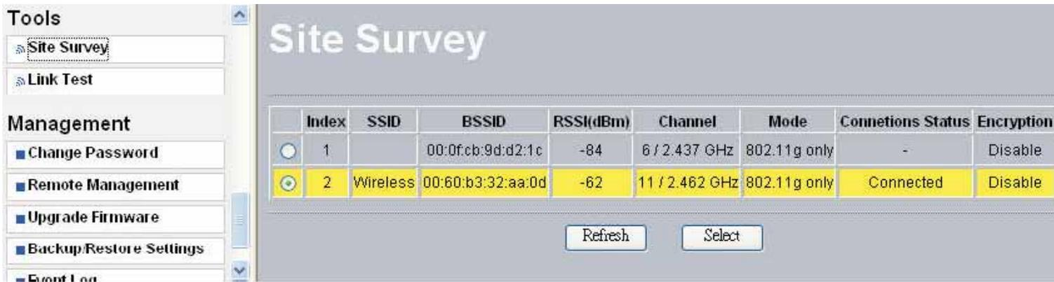
The screenshot displays the LANPRO web interface for the Site Survey tool. On the left, there is a navigation menu with 'Tools' and 'Management' sections. Under 'Tools', 'Site Survey' and 'Link Test' are listed. Under 'Management', options include 'Change Password', 'Remote Management', 'Upgrade Firmware', 'Backup/Restore Settings', and 'Event Log'. The main content area is titled 'Site Survey' and features a table with the following data:
