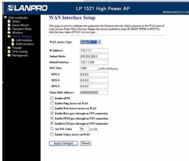
Screen snapshot – WAN Interface Setup – Static IP Figure 23
