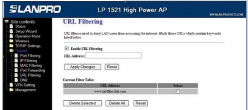
Screen snapshot – Firewall – URL Filtering Figure 31
