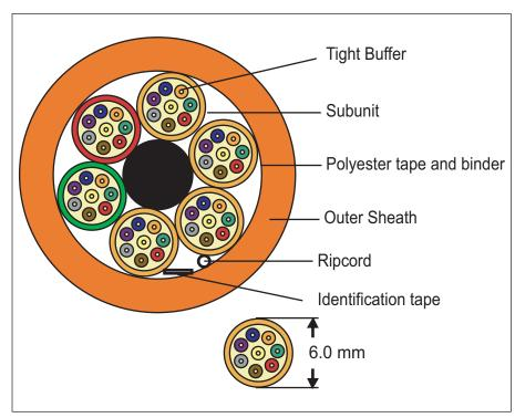
Tight buffers are put into the subunits or simplex tubes that are made of fire retardant PVC material. These subunits are colored for identification and are stranded around a central strength member. Aramid® yarns are put into the subunit for giving cushion to the tight buffers and for giving extra pulling strength.
