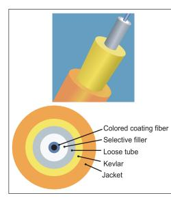
Loose tube material is usually poly butylenes terephthalate (PBT).
