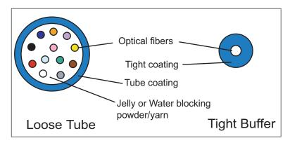
In loose tube coating, the fibers are free to move inside the tube which is filled with jelly or water blocking powder or Aramid® yarn.
