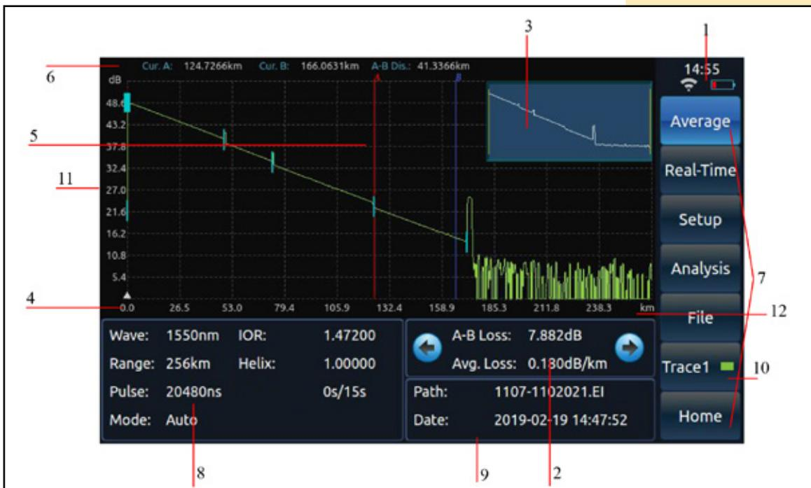
**Fig. 3-1 Diagram of LPT-OTDR70 testing interface**
