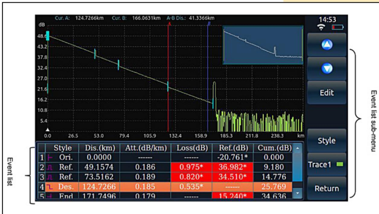
Fig. 3-2 Diagram of LPT-OTDR70 analysis interface
