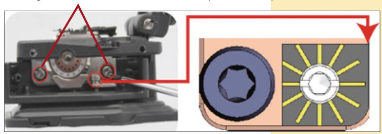
In order to change the height of blade, rotate the M3 screws (Right screw). Rotate screw to clockwise to make it higher and counterclockwise to make it lower. Use HG-78 (Blade Height Adjustment Gauge) to adjust the height of blade. Make sure to clean the cleaver according to this manual instructions ("Cleaning the Cleaver") before using HG-78.
