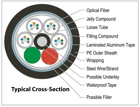
The water blocking tape is for fiber count of 98 to 144 only
