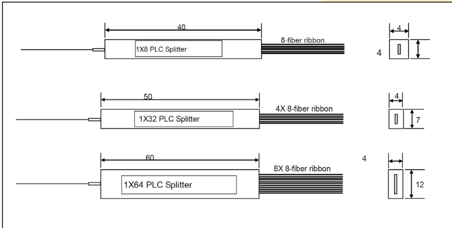
**PLC Capsule Module device Loose Fiber**
