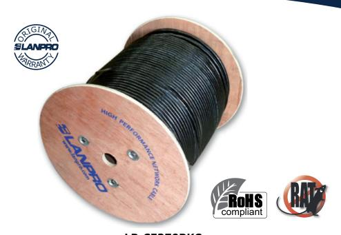
LP-CE370BKC LanPro Reliable® CAT 5E F/UTP Outdoor Network Cable, solid AWG 24 100% copper, Aluminum over Mylar® Foil shield with drain wire, Double Jacket (Black PE plus Gray CMX) and ripcord in a 1000 ft (305m)wood spool.
