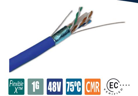
LP-C6320BLC LanPro Reliable® CAT 6 type F/UTP Shielded Network Cable, CMR-rated with Solid Copper Conductors and Flexible-X™ separator for symmetry and Blue jacket, packed in a 1000 ft (305 m) wood spool.
