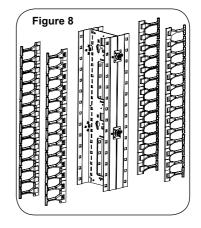
3.3 Slide (6) door hinges over the edge of cable tray door and install door panel on the cable guides.
