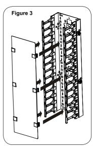
Align the mounting buttons with the mounting slots and then slide the cable tray downwards until secure (2 Post is shown above, same steps for 4 Post).
