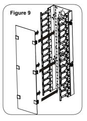
3.4 Align the mounting buttons with the mounting slots and then slide the cable tray downwars until secure. (2 Post is shown above, same steps for 4 Post).
