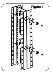
Attach (28) cable guides to the cable tray frame, the cable guides slide over the edges of the cable tray frame to form a tight attachment.
