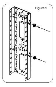
Attach (14) cable guides to the cable tray frame, the cable guides slide over the edges of the cable tray frame to form a tight attachment.
