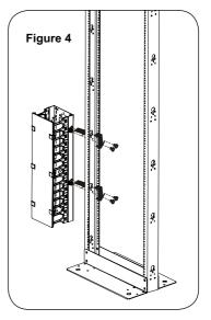
2.5 Repeat Steps 1-4 to assemble and mount the other two cable trays, then using (2) tie plates and (8) M4x8mm screws to connect adjacent cable trays for added stability.
