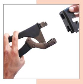
2.- Press the button at both sides while pushing the body on to the head with the Die until securely fixed.
