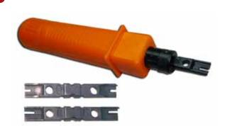
The LanPro **LPT-314BK**, a very durable and reliable tool, also named 110 or Kröne punch down tool, with a traditional design, is a hand-held impact tool that helps the telecommunication technician to terminate structured cabling connectors with insulation displacement like punch down blocks, keystone compatible jacks, or patch panels with IDCs of the 110 or Kröne standard.
