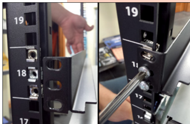
Figure 16 Left sliding bar bracket fixation
