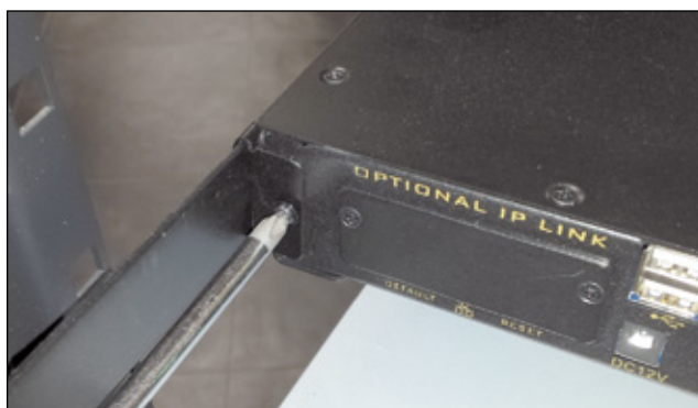
Figure 21. Fixing of the left lateral adjustable bracket to the back of the KVM.
