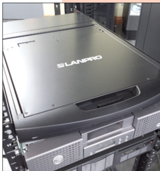
Figure 20. Shows the KVM from the front of the rack before fixation to the rack's vertical rails.
