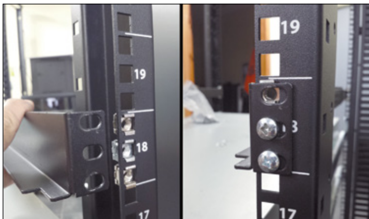
Figure 17. Right sliding bar bracket fixation.
