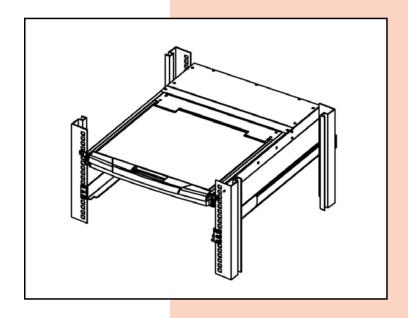
3 Slide the rear attachment sliding brackets along the slide bars until they contact the rear of the switch.
