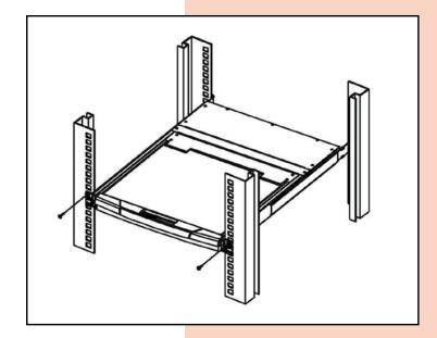
4 Use the screws supplied with this package to attach the bars to the rear of the switch.
