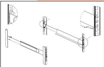
6 Place the KVM Switch in the installed bracket and secure the KVM Switch, cabinet and mounting bracket.
