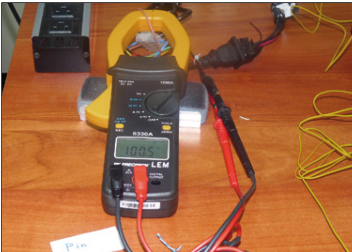
Figure 4. Input AC Voltage measured: 100.5 VAC
