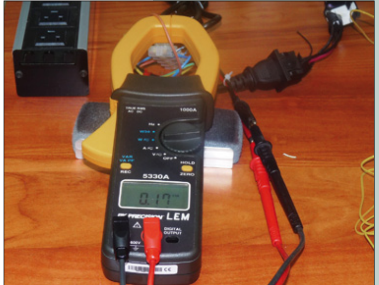
Figure 7. Apparent Power measurement is 0.17 KVA
