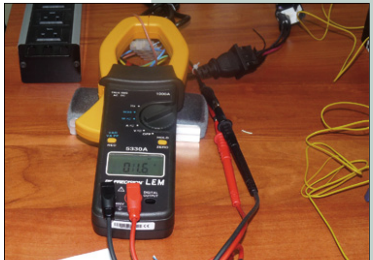
Figure 5. Line Current Amperes read: 1.6 Ampere AC
