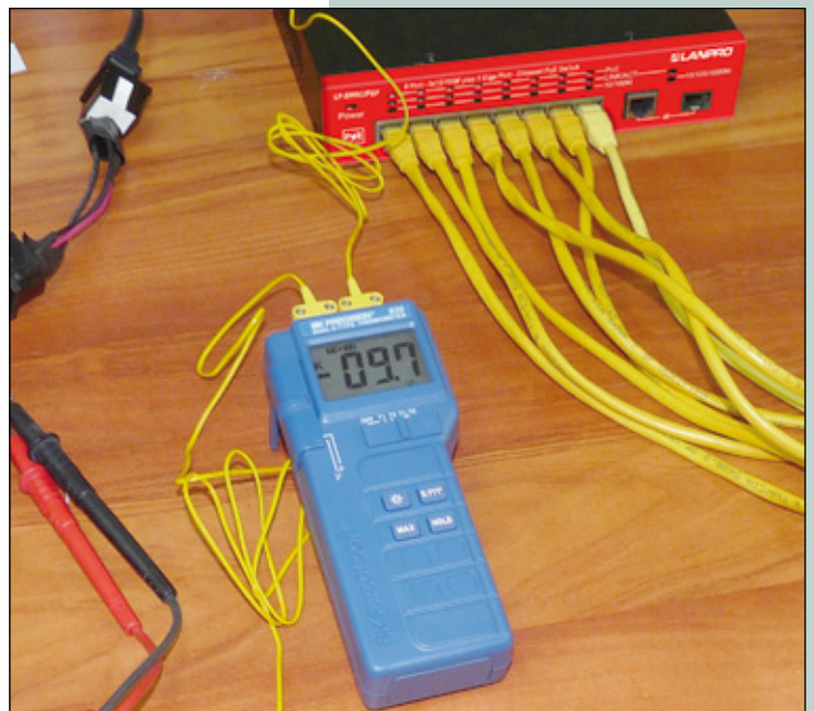
Figure 9. Temperature differential after 4 hours= 9.7°C
