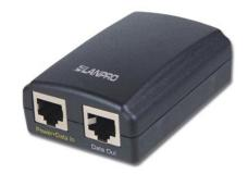
The LP-Poe151 PoE Splitter is designed to supply operational power to surveillance cameras and wireless LAN devices such as access points, bridges and routers. It enable power current to travel on the Ethernet network cable, thus eliminates the need to directly connect a power supply to the wireless LAN device. It can be utilized to support voltage from 18V to 55V or comply with 802.3af standard by switch.
