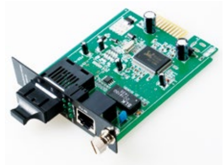
Media Converter card version for chassis mount
